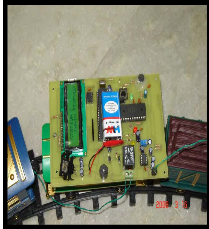
Fig.8. PCB mounted on the engine of the train.
