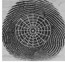
Figure 2. Reference point (x), the region of interest and sectors superimposed on a fingerprint
