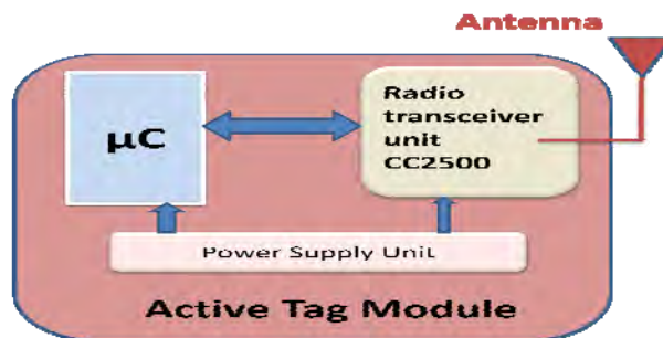
Figure.2 Block diagram of active tag module
