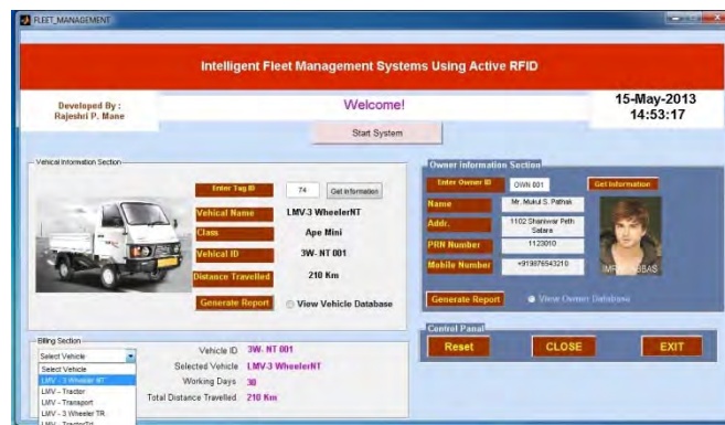
Figure 5 GUI for Intelligent Fleet Management Systems Using Active RFID
