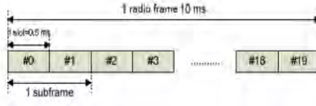
Figure 1. LTE time-domain structure
