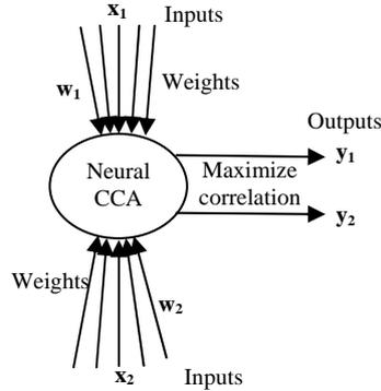
Fig. 2: The CCA network for correlation determination between two sets of EEG data.
