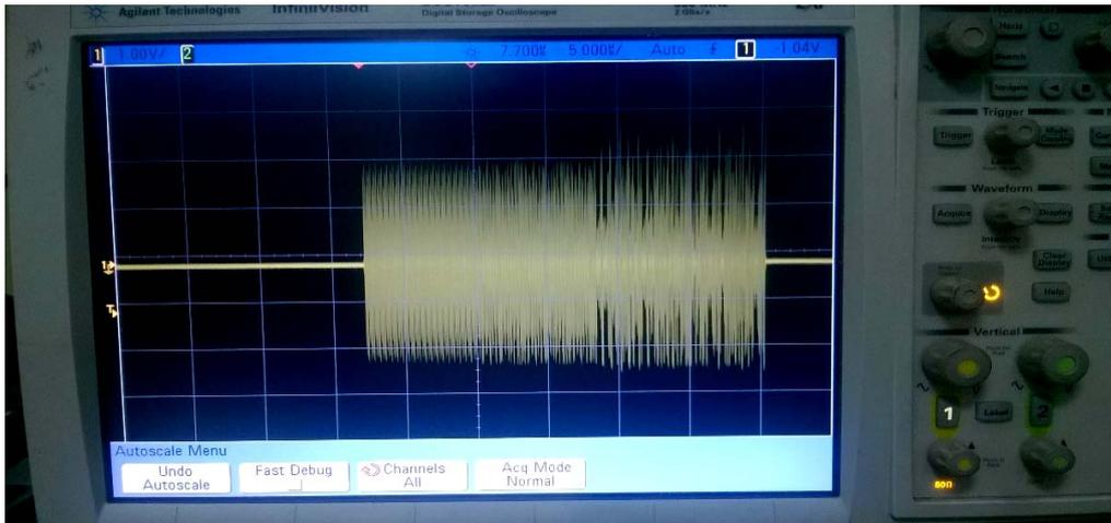
Figure 15. Received signal in time domain on DSO7032B
