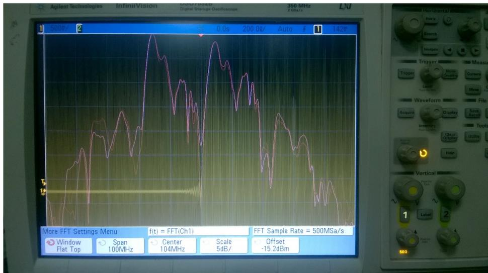
Figure 19. Signal spectrum in Flat-Top Window
