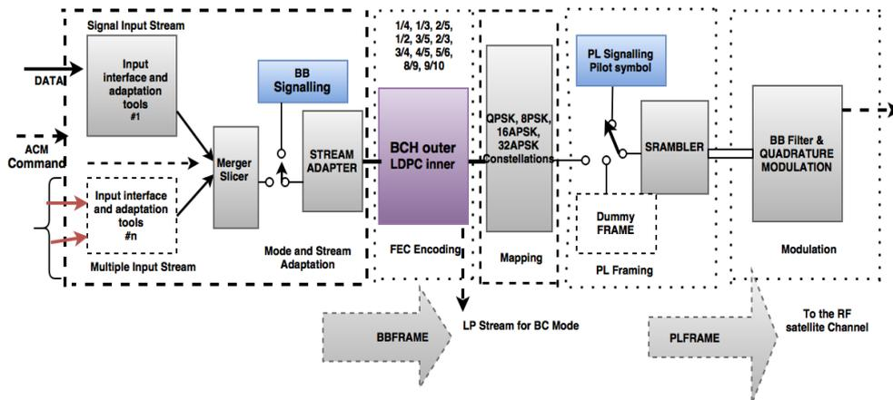
Figure 7. DVB-S2 Transmitter Block Diagram
