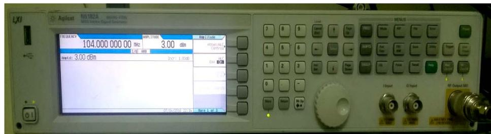
Figure 14. Wi-Fi n signal dumped in Agilent MXG
