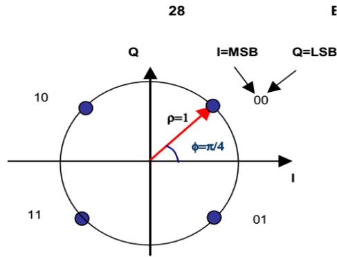
Figure 3. Bit mapping into QPSK constellation
