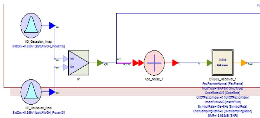
Figure 10. Addition of Noise Signal
