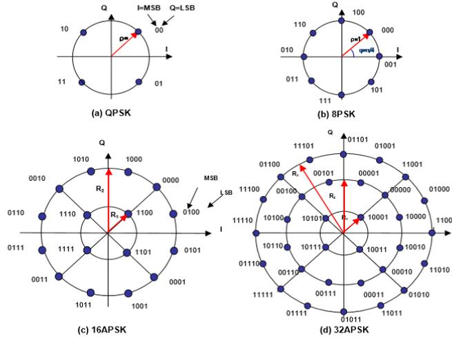
Figure 2. The four DVB-S2 constellations QPSK, 8PSK, 16APSK, and 32APSK before PLScrambling.
