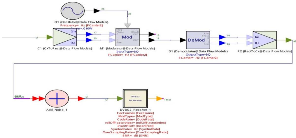
Figure 9. Implementation of Carrier Frequency Over Signal
