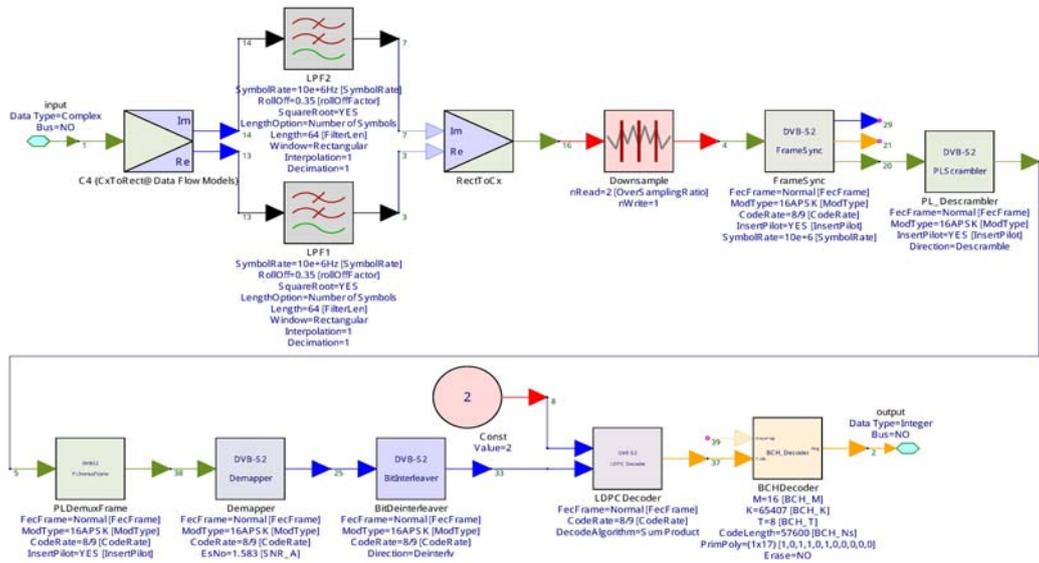
Figure 11. DVB-S2 Receiver Simulation Design
