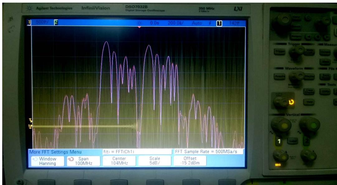
Figure 20. Signal spectrum in Hanning Window
