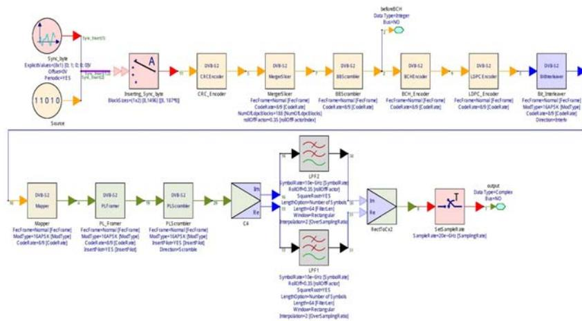
Figure 8. DVB-S2 Transmitter Simulation Design
