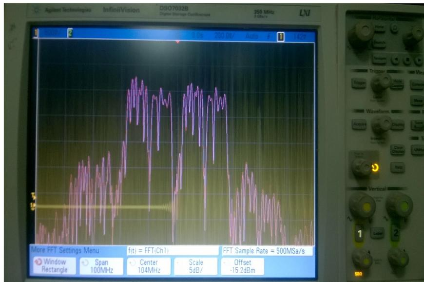
Figure 17. Signal spectrum in Rectangular Window
