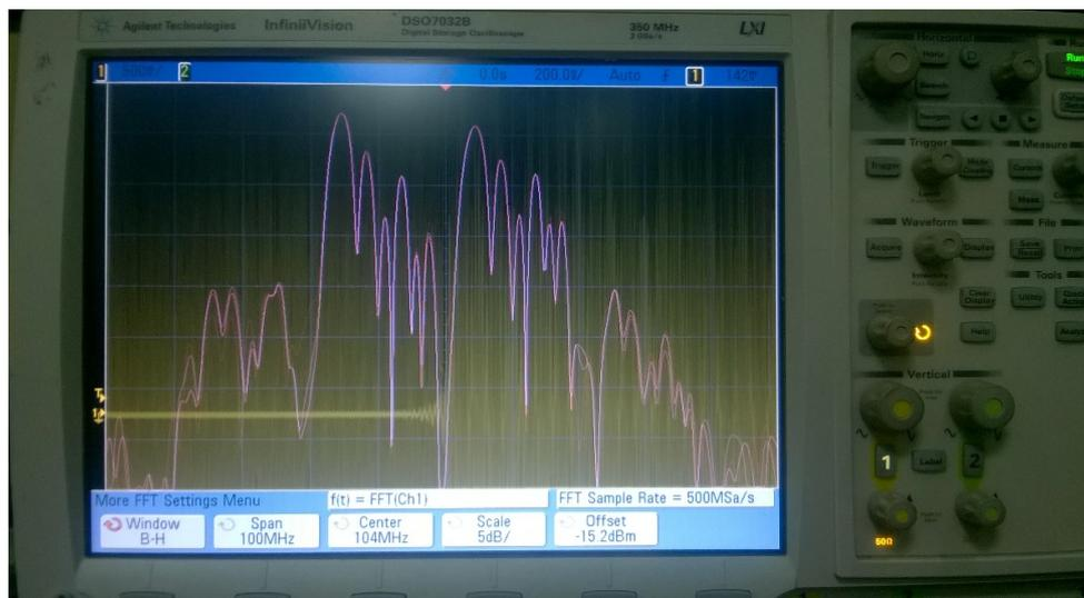
Figure 18. Signal spectrum in Blackman-Harris Window
