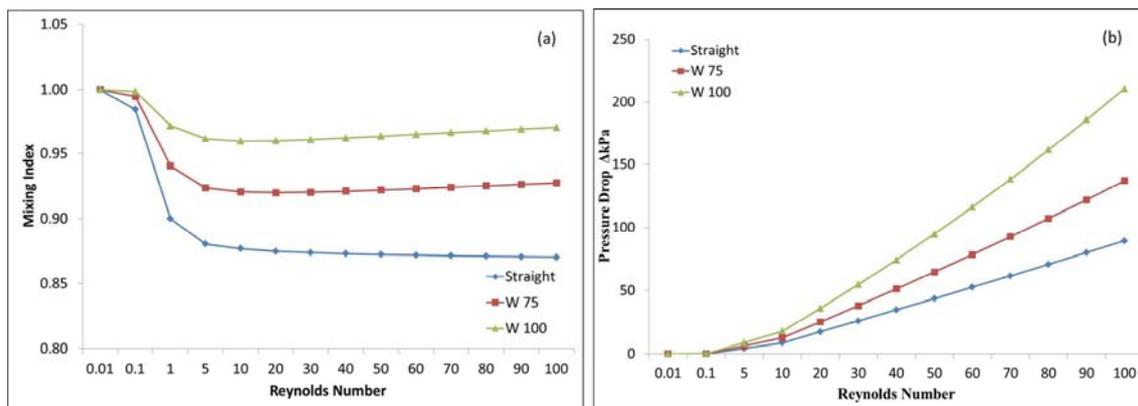
Figure 5.(a) Comparison of Mixing Index of Straight, Wing-75 and wing-100 micromixer; (b) Comparison of Pressure drop of the same; both using mesh M1.
