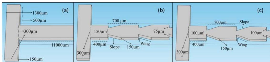
Figure 1. Geometry of (a) Straight, (b) Wing-75, and (c) Wing-100 micromixers.
