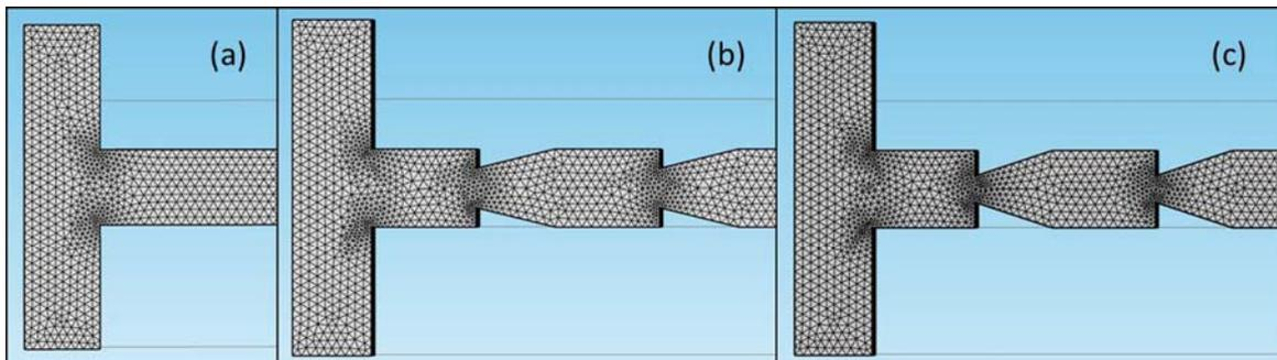
Figure 3. (a) Straight, (b) Wing-75, and (c) Wing-100 micromixer mesh M1.
