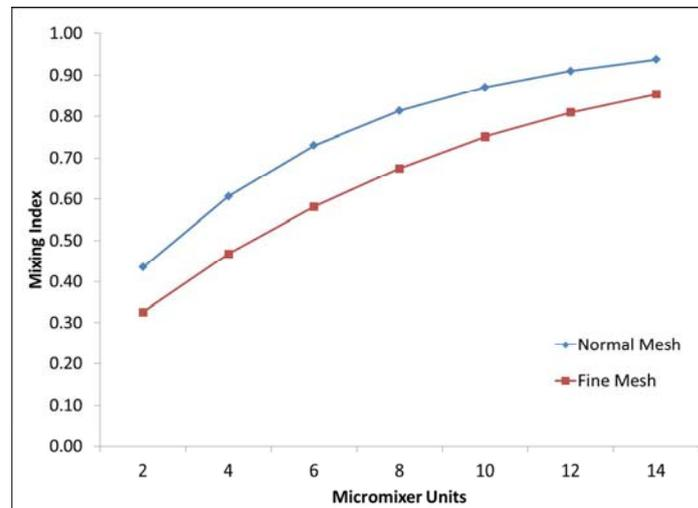
Figure 9. Mixing Index of Wing-100 micromixer with mesh (M2 and M3) at different units at Re 60.
