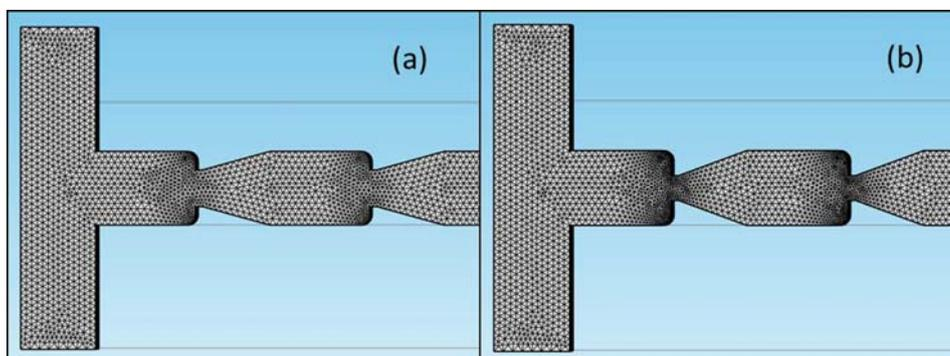
Figure 4. The refined meshing of (a) Wing-75 and (b) Wing-100 micromixer using mesh M2.
