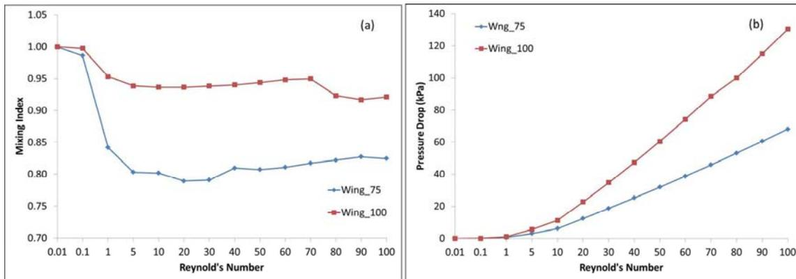
Figure 6. (a) Comparison of Mixing Index of optimized Wing-75 and Wing-100 using mesh M2 and (b) Comparison of Pressure drop for the same.
