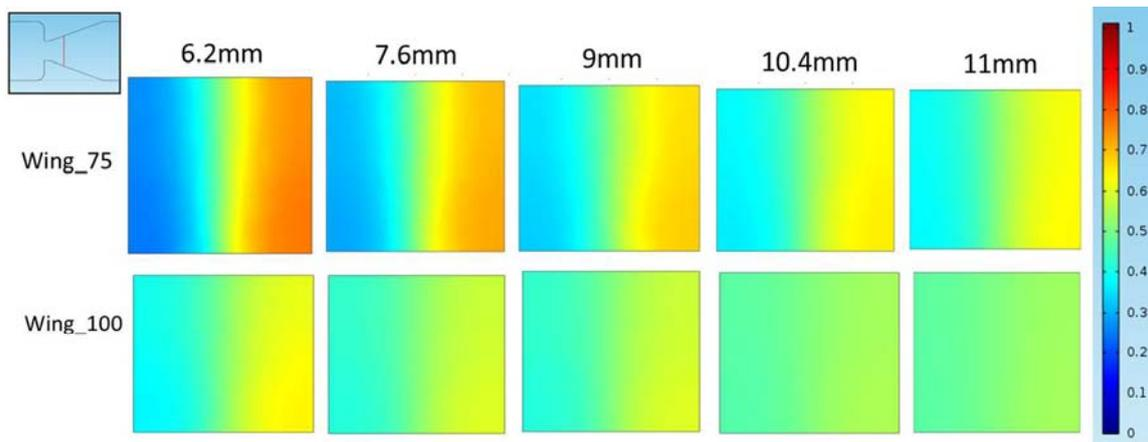
Figure 8. Concentration gradient of mixing fluids (Re 60) at different values of axial length in Wing-75 and Wing-100 micromixers.
