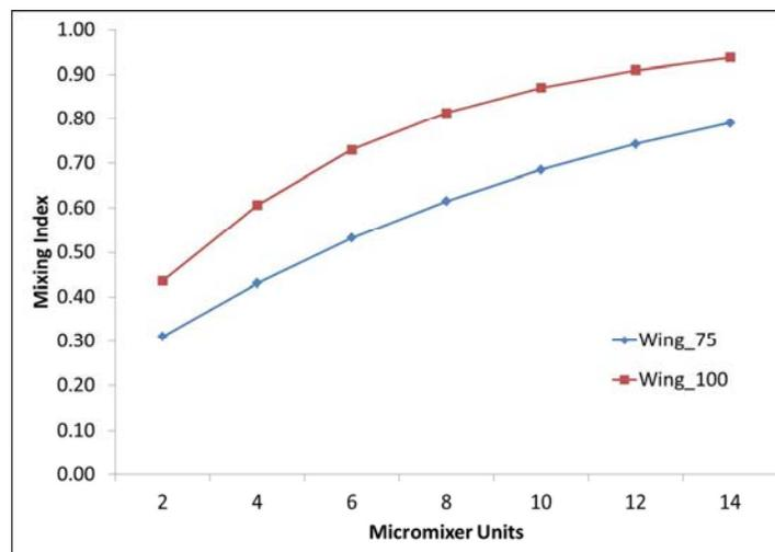
Figure 7. Mixing Index at different units of the Wing-75 and Wing-100 micromixer at Re 60.
