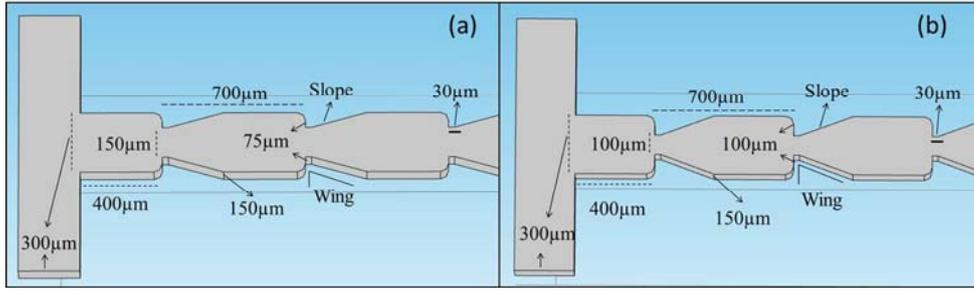
Figure 2. Geometry of (a) Wing-75 and (b) Wing-100 micromixers with flattened wing tip and rounded outer corner.
