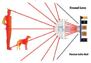
We developed a human tracking system using a sensor cluster consisting of sensors and Fresnel lens arrays to implement the desired spatial segmentations. This solution was found out to be the most promising and reliable for applications of this robot.
