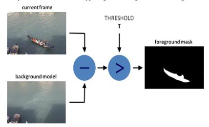
After subtracting the current frame from the background image, foreground mask is generated using the motion depth values. Foreground mask is nothing but a binary image containing pixels that belong to the moving objects appearing in the camera. As soon as motion is detected our robot will send a set of images to the owner as an intruder alert.
