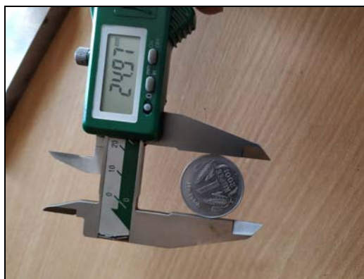
Figure 3. Showing real dimensions of reference object (a standard Indian one-rupee coin) which is 24.97 mm
